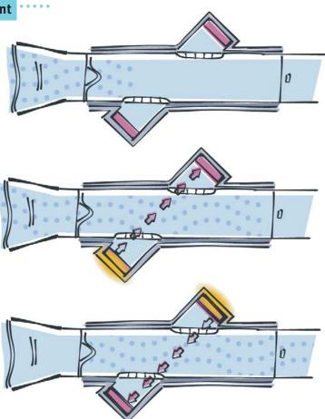
Transducers located on either side of the spirette™ cavity emit and receive sound in alternating directions.
